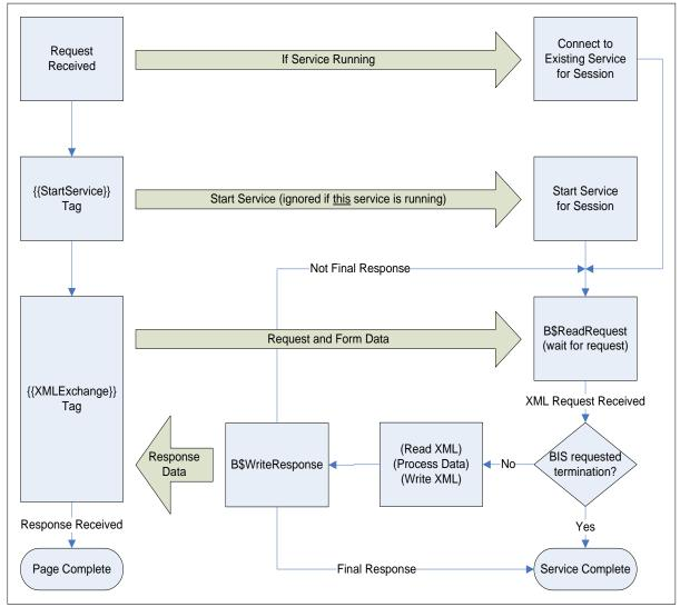
Figure 6-1. BIS Control Flow.
