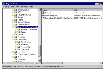
The SourceBridge installation also adds registry keys to the **Local Machine\Software\TeamShare\SourceBridge** folder, as shown in the following figure. The **UnderlyingSCC** key points to the source control provider that is intercepted by SourceBridge.
