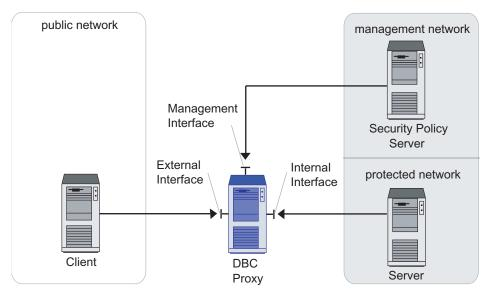
Figure 26 DBC Proxy Network Interfaces
