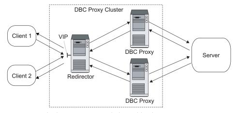
Figure 10 Multiple I-DBC Proxies, balanced load
