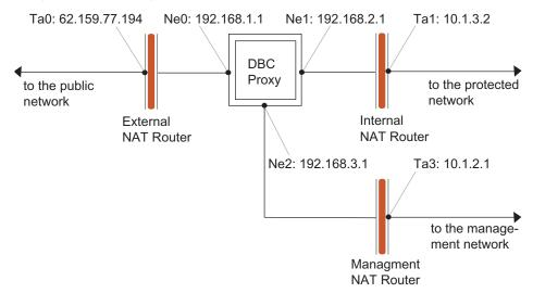
Figure 27 DBC Proxy Network Interfaces
