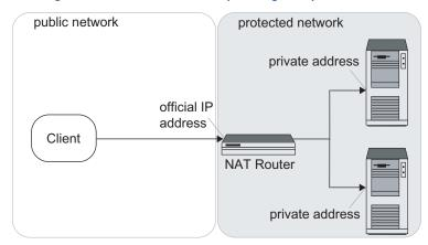
Figure 8 Asymmetric NAT Mapping: The client is located in the public network
