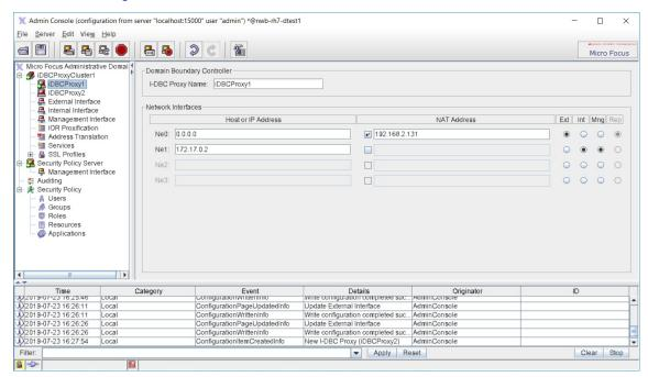
Figure 28 Example for DBC Proxy network interfaces
