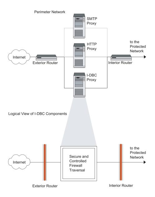
I-DBC Components in a typical deployment Scenario
