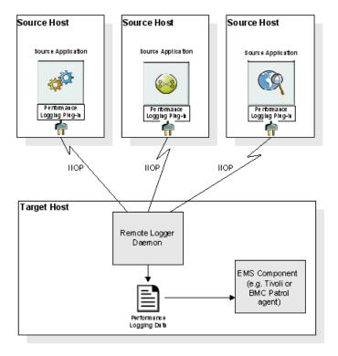
Figure 1: Remote Logging Framework
